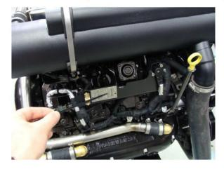
Engine identification tag is located on the starboard side of the engine as shown in photo above.
