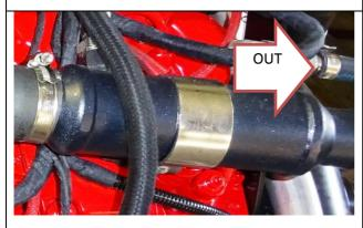
Some configurations with outlet fuel cooler.
