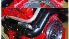
Picture show the exhaust manifolds.
